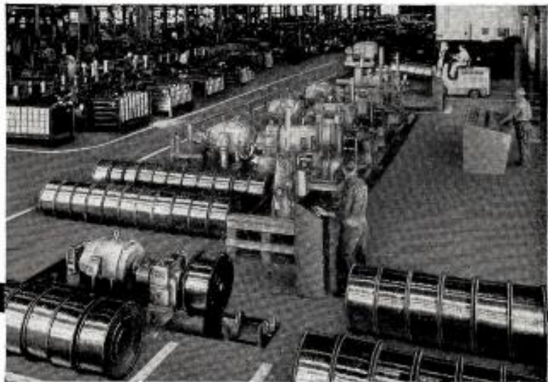
New 3-Stand High Speed Tandem Flat Wire Rolling Mill recently installed at the Ansonia Wire Mill, Ansonia, Connecticut. This mill operates at speeds up to 2000 feet per minute, and is capable of producing 1000-pound reels of finished wire.
