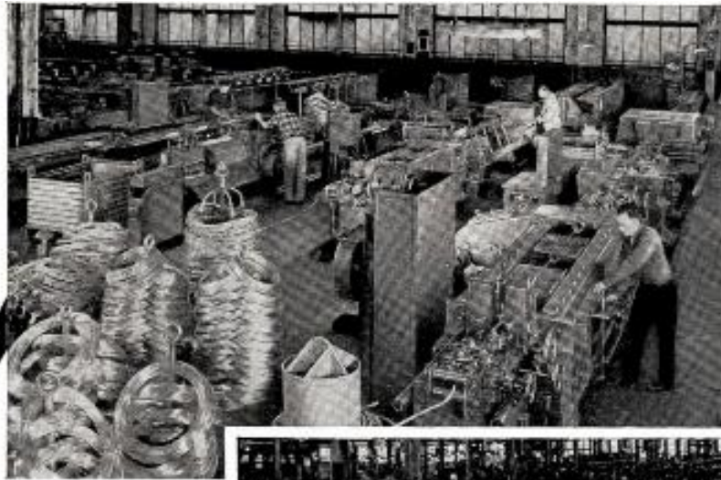
← These modern "four-in-one" Schumag Machines at the Torrington Rod Mill, Torrington, Connecticut produce finished rod in diameters from 3/32" to 7/8". They will finish, draw, cut to length, straighten and polish in one continuous operation.
